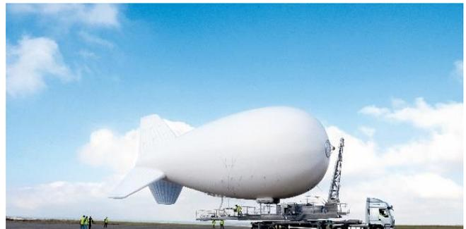
*Condor tethered aerostat © CNIM Air Space*
