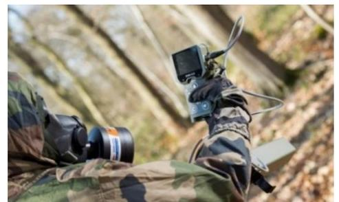
*Multiprobe survey meter SaphyRAD MS
